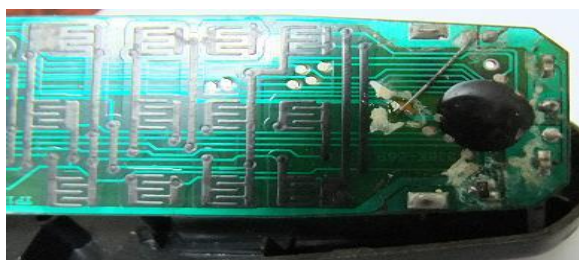
Figure 4. Photomicrograph of a PCB of remote control of TV.
