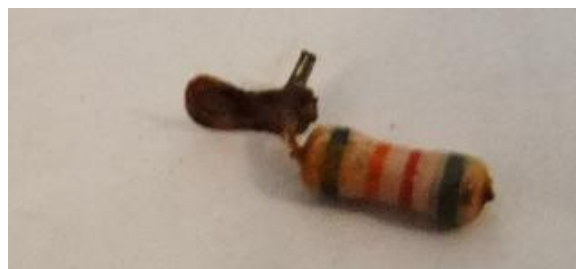
Figure 10. Corrosion at joints
