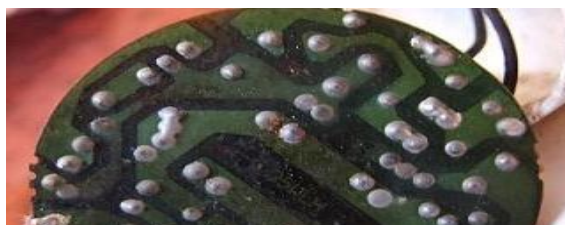
Figure 3. Photomicrograph of a PCB of CFL
